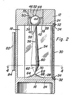
The foreign patent from England GB7203 from **1903, Theodor Hillmer** shows a floating plumb bob used in earth drilling equipment to show and register the inclination of the bore hole.
