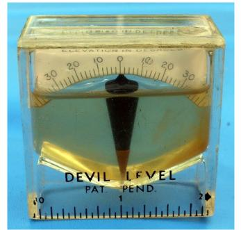
At the bottom the container is triangle shaped to put it on a pipe.
