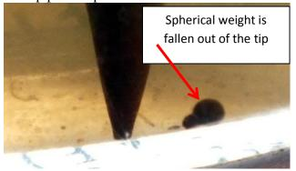
The weight holds the devil in the V-shaped bottom of the instrument.
