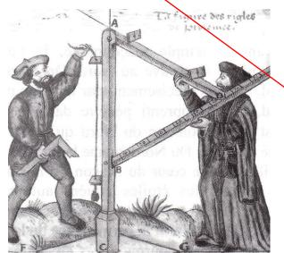
On the horizontal part we find two simple sighting devices. When the iron tip is pressed into the earth down to the beginning of the marking, the horizontal part is 1 meter above the bottom. Now you can use it as a surveying leveling instrument (best position for the surveyor is sitting). The drawing below left shows a similar instrument from the 16<sup>th</sup> century.
