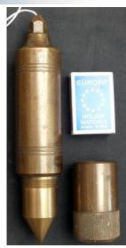
(Fig. left) And a 90 degree mirror with inserted plumb bob for surveyors.
