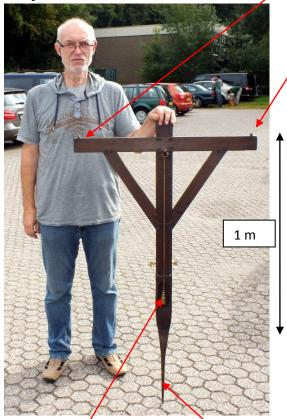
It is a very early measuring instrument for surveyors. It is an inverted A-level combined with a vertical rod. The rod has an iron tip. A plumb bob is fixed at the top to verify the vertical position when the rod is pressed into the earth. On the rod is a scale of 1 meter.
