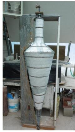
lathe framework which turned against a steel template until it achieved the designed profile. The final coat was smoothed and a clear sealer was applied.
