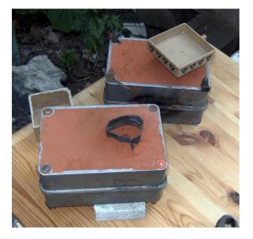
Brass + special chemicals heated to 1000 + degrees Celsius in a graphite crucible and poured into the mould.
