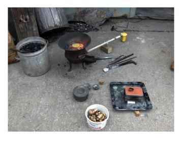
The mould with the model. Upper and lower part. Special casting sand was used.
