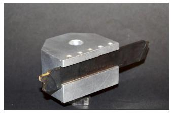
tool post mounted form tool allows me to make small beads or other profiles
