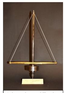
A shop made pump drill made just for fun from the chuck and spindle of a burnt out dremel tool and a length of polished steel rod that came from a discarded ink jet printer. The cross bar with tapered ends and ball details were turned from a piece of 3/4" brass bar stock before the flats were milled on the top and bottom surface.
