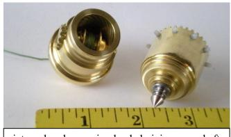
internal reel on spring loaded pinion gear shaft
