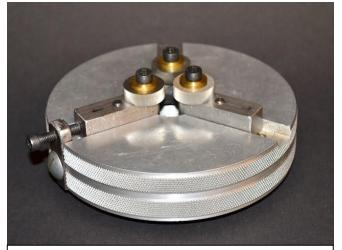
tailstock mounted knurling tool with 3 knurls used to knurl small diameters without having the work deflect from the force applied by ordinary knurling tools that only use two or even just one hardened steel knurl
