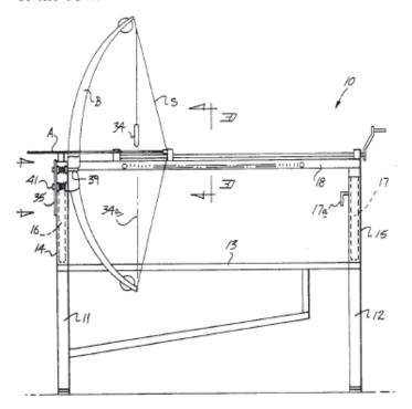
A plumb bob and support line 34 (see FIG. 10) are sighted along a setting line 34*a* to intersect upper and lower terminal ends of the bow "B". To permit vertical adjustment and positioning in alignment of the sighting line 34*a*, a bow mounting plate 35 includes (see FIGS. 5,
