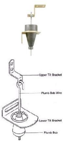
Basically it is a piece of string that is attached to a weight at one end, while hanging from the other. This gives you a perfectly vertical line that is vertically level.
