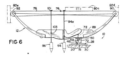
arrow 82 is to traverse. Plumb bob 94 indicates the precise vertical position beneath main bow string 78. With this as a guide, the user then adjusts arrow shelf 84 15 (FIG. 7) laterally (i.e., inwardly or outwardly from the body 89 of bow 12), until the track portion 95 is directly aligned with the string 94a of plumb bob 94.
