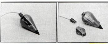
Marked: TROUGHTON & SIMMS Ltd, LONDON Patent No. 6247. Weight is 11 ounces, length 3 5/8". Un-screwing the cap allows the pulley to slip out of the body, which I beleive was only a manufacturing convenience. The width of the pulley is greater than shoulder of the bob so the string only touches the pulley. Somewhere along the line a hole was drilled in the cap to facilitate 'normal' use.
