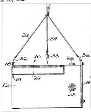
This invention relates to a device for locating the center of gravity of footgear for use primarily, although not exclusively, by members of the Armed Services.
