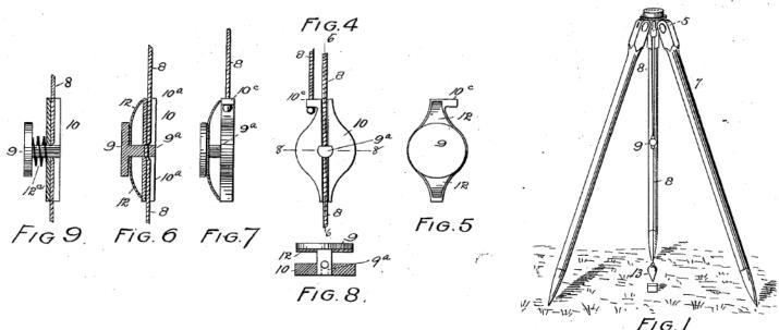
My invention relates to improvements in plumb-bob attachments specially designed for use by surveyors and others who use a plumb-bob in connection with the tripod. By means of my attachment the plumb-bob 20 is readily adjustable.
