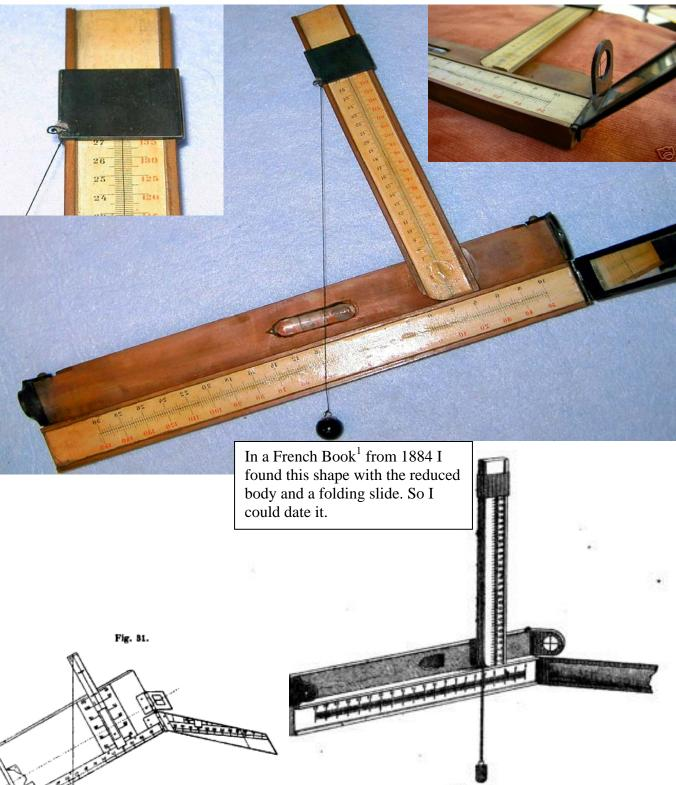
(Fig. left) In 1887 and 1912 was mentioned a modified version<sup>15</sup>. The sighting device is directly above the mirror.
