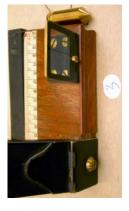
From a Hartmann & Braun 1890s. The plumb bob in its "garage". The scale with division markings in "Strich" (black) and "Meter"
