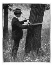
FIG. 63.—Calipering a tree.
