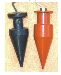
Fig. 36. Surveyors plumb bobs powder coated.
