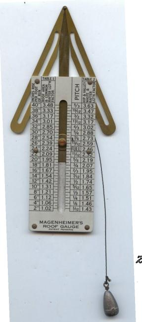
**USE OF ROOF GAUGE** 1. Find pitch of roof, Fig., 1, by holding gauge vertically and adjust blades to member with roof lines. Read pitch on scale at indicator.
