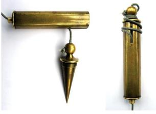
a small, one piece, solid brass construction that screws into a brass tube for protection - everything normal to this point. Furthermore, the tube has a slit at the open end which allows the exit of the line, but this is impractical, because the line is twisted and tangled when the plumb bob is screwed into place. There is also a threaded opening at the closed end of the tube, with something possibly missing.
