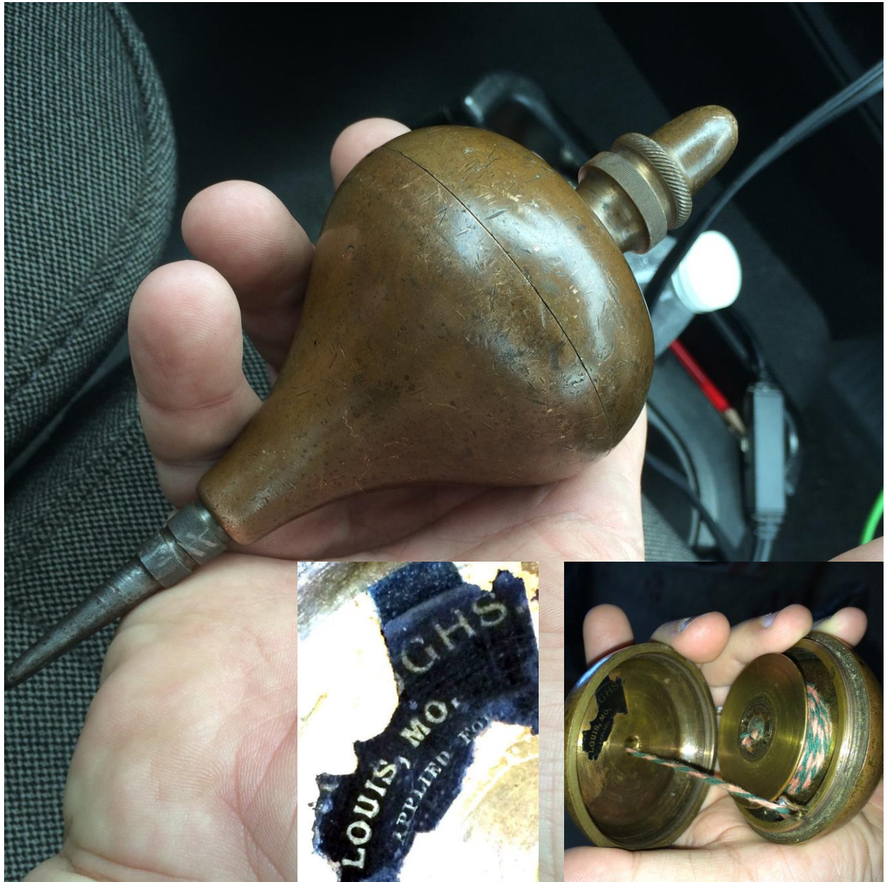
Unknown mechanical plumb bob made in St. Louis, MO, U.S.A.. 2.8 lbs; 7 in tall; 2.8 in diameter. (More see my Newsletter 2015-Q 04)
