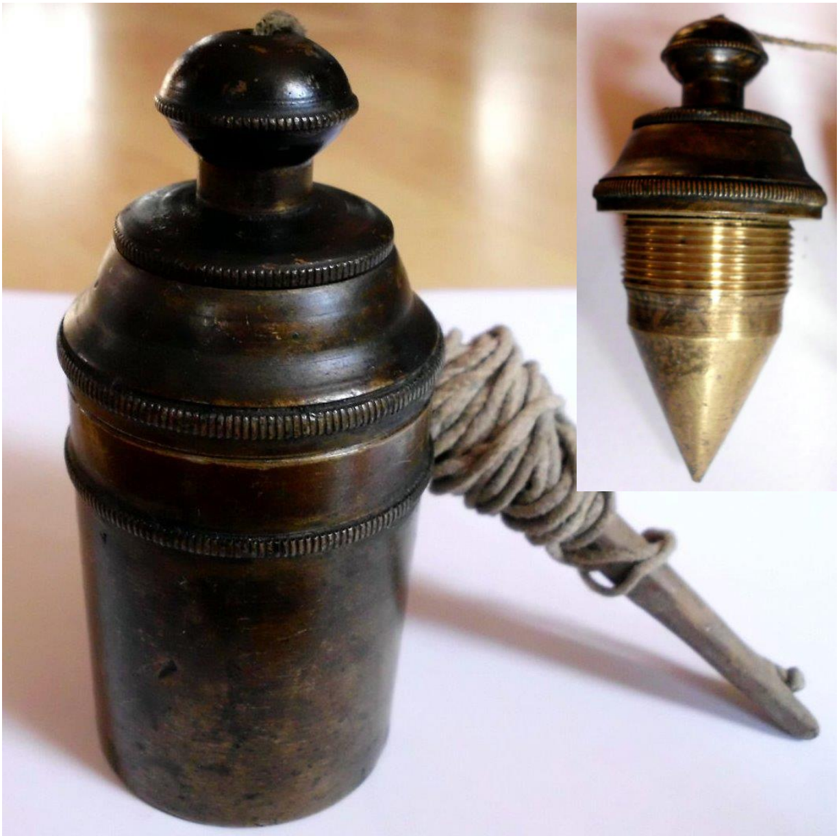
German brass plumb bob. 4 ¼ in high; 1 ¾ in dia. (More see my Newsletter 2015-Q 05)
