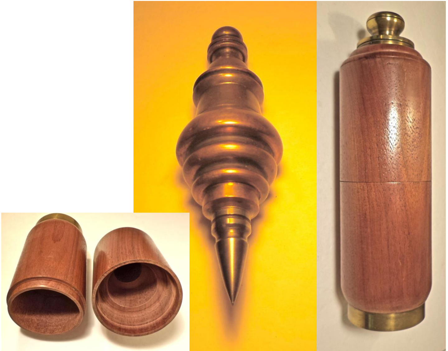
Plumb bobs made by Herb Kean, Morristown, NJ, U.S.A.. Solid brass 8 ½ inch long. It weighs 5 ½ pounds, the container 3 pounds. (More see my Newsletter 2015-Q 03)
