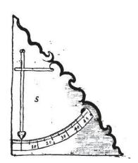
This is for the cross slope / transverse inclination (scale +/- 10 degrees)
