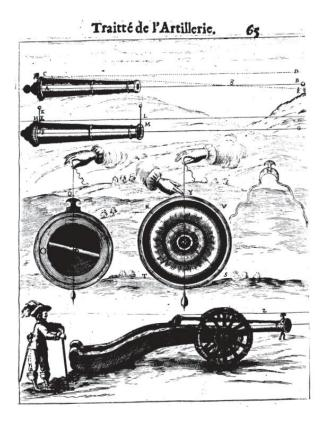
The manufacture of cannons in the 1600s posed many difficulties. The walls were different thick and the axe of the tube was not in the middle of the barrel. Proper placement of cannon sights required very specific positioning.
