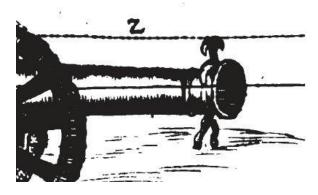
To make certain the artillery soldier located the position of the sight exactly OVER THE MIDDLE of the barrel (center, axe) they used the plumb bob and a small wooden stick. ©
