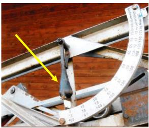
On the scale you can find the DEGREES, LENGTH of the ladder and the resulting MAXI LOAD.
