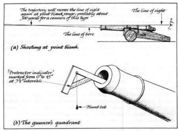
Fig. 8 Shooting at point blank and the use of the gunner's quadrant NOTE. Aiming 'by the line of metals' at a target level with the gun results in a positive angle of elevation of the bore of the gun of 1-3°, depending on the geometry of the gun.
