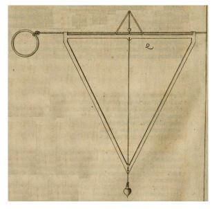
It looks a little bit different and has a second plumb bob on top. The author Daniel Speckle did not mention that it hung between two rods without tension (not pulled by hand, but hanging loose in the middle of the line). The one depicted appears to show that the line was tightly stretched by hand by pulling rings. We see that this instrument was used in Europe in different countries at that time.
