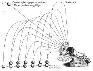
Figure 4 (left) is a gunner's quadrant that divides the 90 degrees into 12 parts (6 parts with 7.5 degrees to each side)
